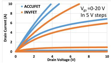
ACCUFETs have better output characteristics and R<sub>on,sp</sub> compared to INVFET due to higher channel mobility and lower V<sub>th</sub>.
