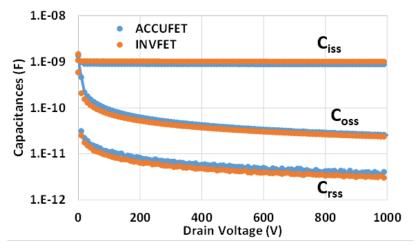
Measured C<sub>iss</sub>, C<sub>oss</sub> and C<sub>rss</sub> are very close for both devices due to same basic cell structure.
