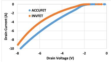
INVFET has higher voltage drop in the 3<sup>rd</sup> quadrant at a fixed value of current due to its higher channel potential.
