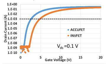
V<sub>th</sub> for ACCUFET is lower than that for INVFET because of smaller band bending required to create a channel in case of an n-type base region.
